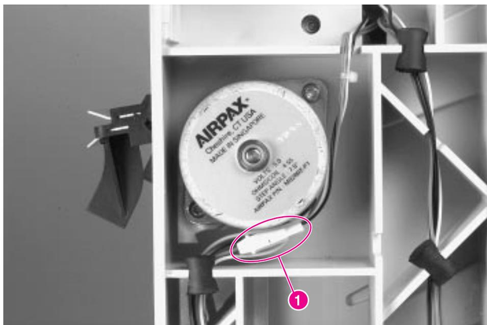
**Figure 6-58** Mailbox with Stapler, Flipper Assembly Connector
